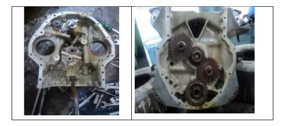
The condition of Oil Pump and housing, Tachometer drive, Vacuum pump drive, Crankshaft gear, Camshaft Gear and Magnetos drive gears were found intact. No damage observed.
